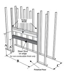
NOTE: Steel stud must be installed after unit has been positioned in place and prior to installation of non-combustible finishing. Steel stud is required for non-combustible finish only.
